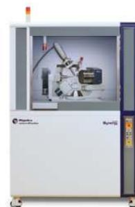
Rigaku XtaLAB Synergy single crystal X-ray diffractometer
